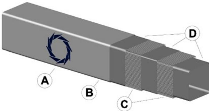
**A. Resin Matrix** - Specifically formulated and dispersed throughout the entire profile (approximately 35% by weight), the resin matrix also includes various additives such as UV stabilisers, Fire Retardant compounds, colour pigments and mould release agents.
