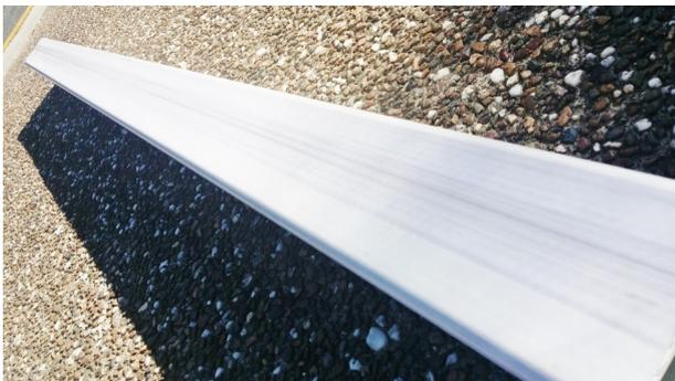
The square tube in the picture (left) has been under constant UV exposure since it was produced, some 30 years ago in the United States. Every year, the sample is load tested to determine if structural properties are diminished from continuous UV exposure. Since initial testing, the profile's colour pigments have almost completely faded, yet the tube has lost less than 1% of its strength (line load tested over 3' span).
